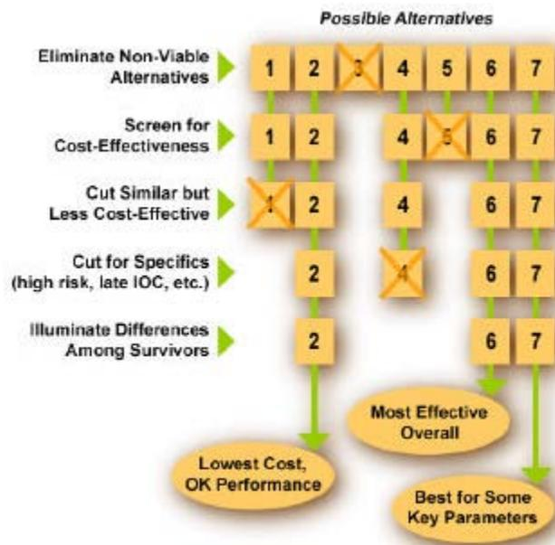
**Figure 5-1: Eliminating Alternatives in an AoA**
